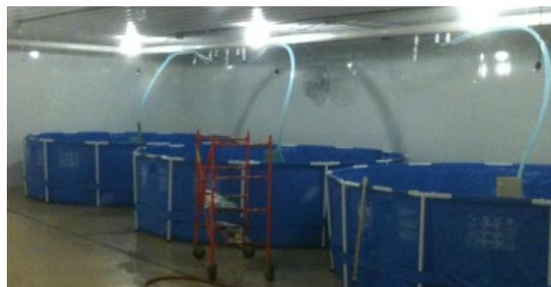
Our system is very simple. It is based on air stones and a pump in a pool of salt water. Can't get much simpler than that? Mother Nature is complicated
