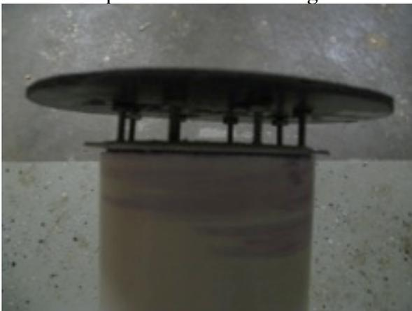
*Top view of drain with antivortex cover before installation.*
